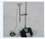
Apart from horizontal movements glacier undergoes the phenomenon of ablation. Ice mass is melting under various conditions (like rain, warm winds, sun rays etc). Traditional method of measurement comes down to reading of ablation scale's current value and comparison with former results. Main flaw of this simple method is influence of melting the pole into ice. Diagram presents comparison of ablation determining using traditional method and GPS determined altitude.
