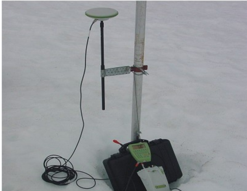
Fig. 3. Ablation pole with GPS antenna (A.Adamek)
