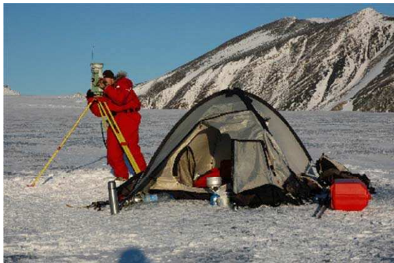
Fig. 12. Hans Glacier movement velocity measurement using Leica Smart Station system (Woźniak and Adamek, 2007)
