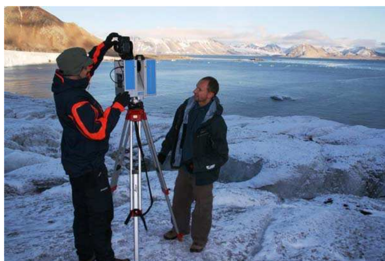
Fig. 14. First test of Z+F Imager 5006 scanner with integrated digital camera on Hans Glacier in 2007. Artur Adamek on the right (W. Krawiec).
