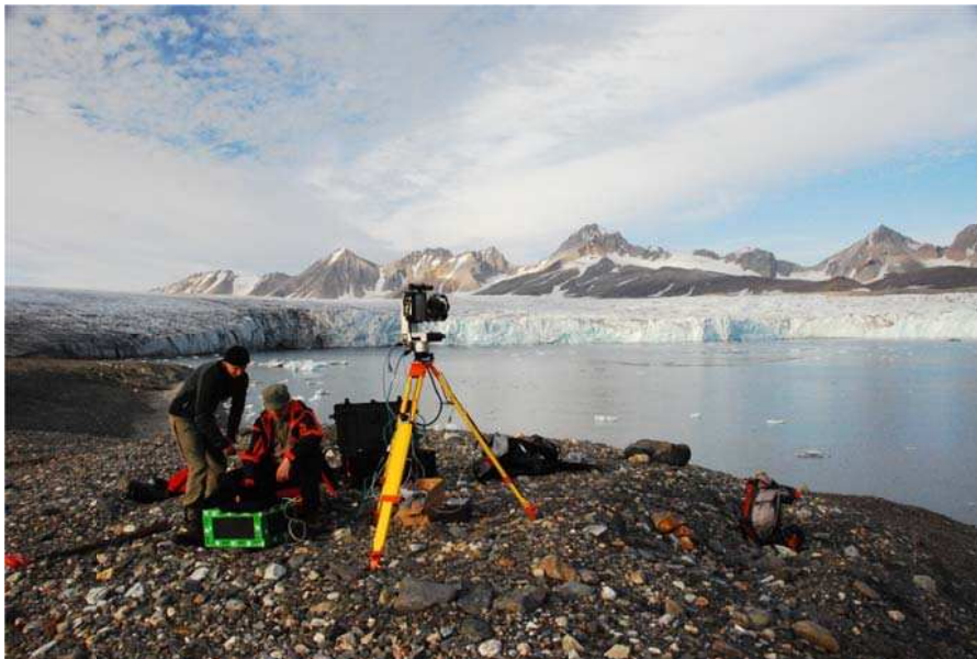
Fig. 15. Hans Glacier scanning using Reigl LPM-321 long range scanner (W. Krawiec)
