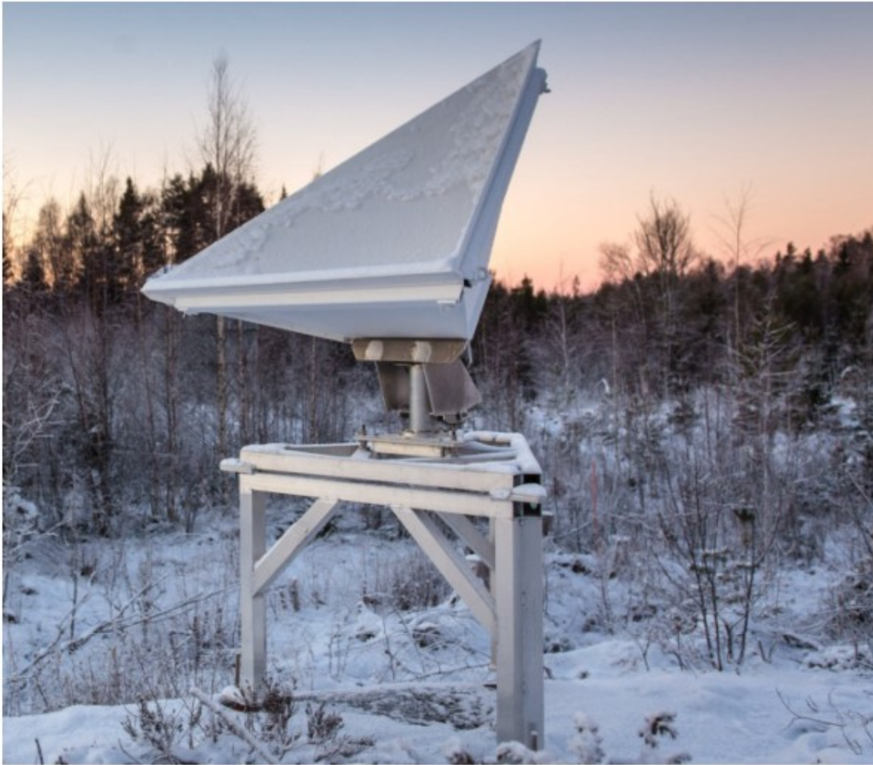
1.5 m corner reflector w Metsähovi (Finlandia) (źródło: Survey Protocol for Geometric SAR Sensor Analysis, 2018)
