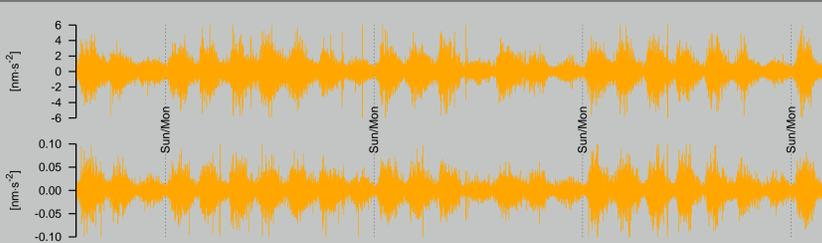
Figure: Time derivative of raw (top figure) and filtered (bottom figure) gravity residuals (tides, ocean loading and pressure effects removed)
